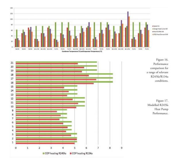
cooling and the use of the buffer tank ensured that satisfactory run times would be obtained under all conditions. Heat exchangers were selected with R245fa and water in mind but the larger expansion valve proved difficult in obtaining R245fa operating values. It was operated with the compromise setting of R123 which was deemed closest to the R245fa pressure/temperature levels.
