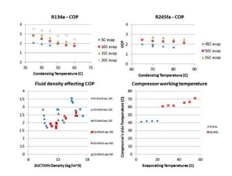
The water to water heat pump was initially tested with R134a at EN14511standards to establish correct operation and a baseline performance. The performance map was the extended to higher temperatures to allow meaningful R245fa tests. Figure 15 illustrates comparative performance between the two fluids.
