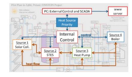
The control algorithm developed for the Polish pilot plant contains a two-level approach. The low level controller is responsible for the implementation of predefined operating modes for heat transfer between different heat sources, heat storages and heat consumers. The high level control is responsible for optimising the overall system performance taking the historical data, current system state and future predictions into account.
