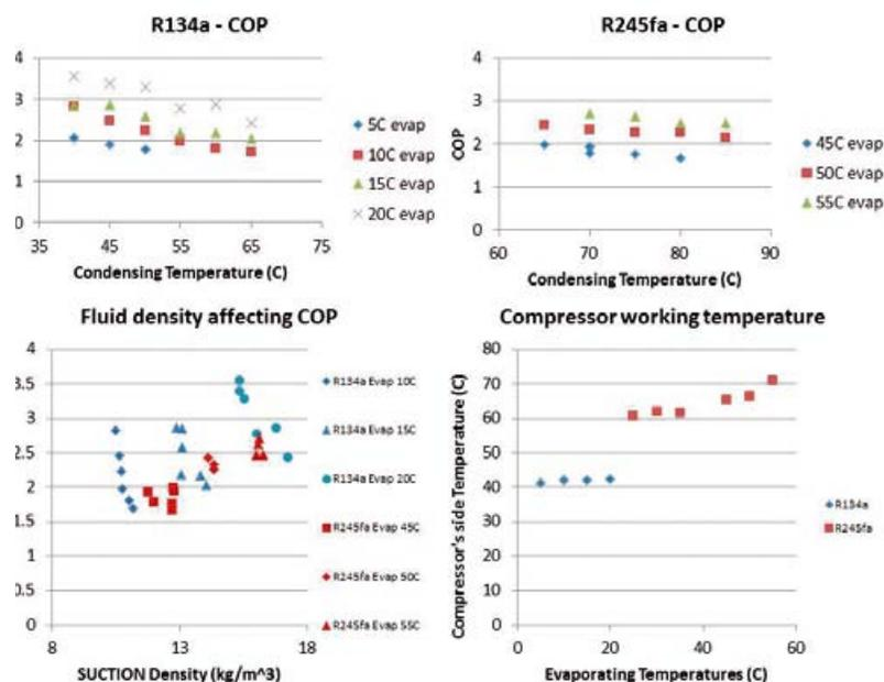
The water to water heat pump was initially tested with R134a at EN14511 standards to establish correct operation and a baseline performance. The performance map was extended to higher temperatures to allow meaningful R245fa tests. Figure 15 illustrates comparative performance between the two fluids.
