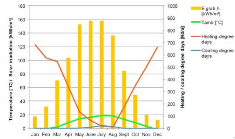
Figure 2. Monthly values for solar irradiation (E\_glob,h), ambient temperature (Tamb), heating and cooling degree days for Warsaw according to Meteoronorm.
