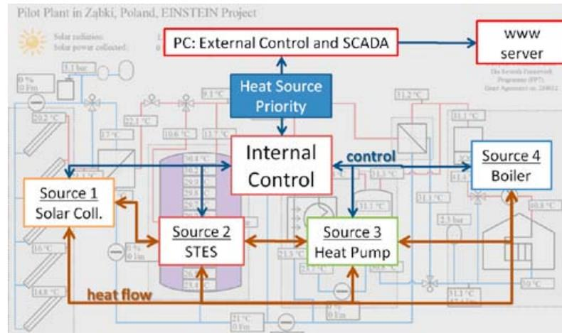
The control algorithm developed for the Polish pilot plant contains a two-level approach. The low level controller is responsible for the implementation of predefined operating modes for heat transfer between different heat sources, heat storages and heat consumers. The high level control is responsible for optimising the overall system performance taking the historical data, current system state and future predictions into account.
