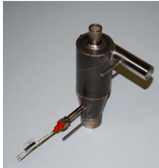
Developed anode Offgas burner
